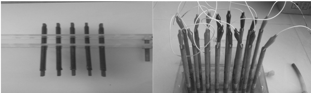
图1 模拟粒子固定及电解槽实物图 Fig. 1 Simulated particle electrode and electrolytic cell
